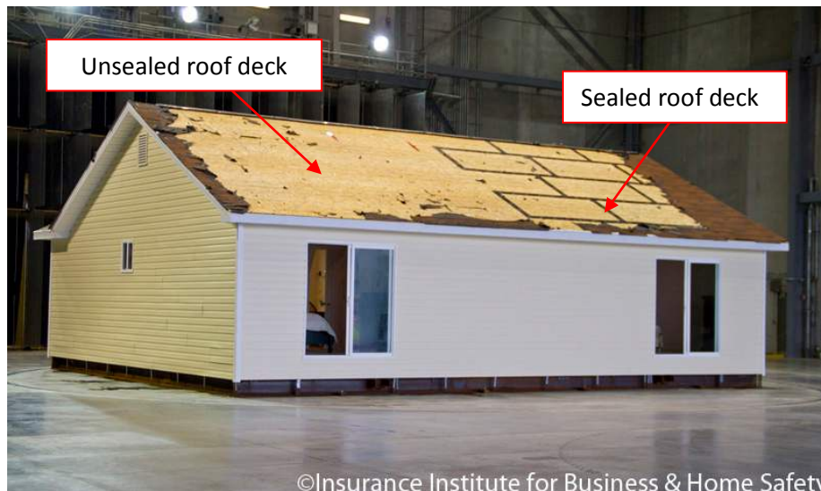
Figure 3. Photograph of the back of the duplex after shingle and underlayment (manual) removal, illustrating the sealed roof deck (right) and the unsealed roof deck (left).
