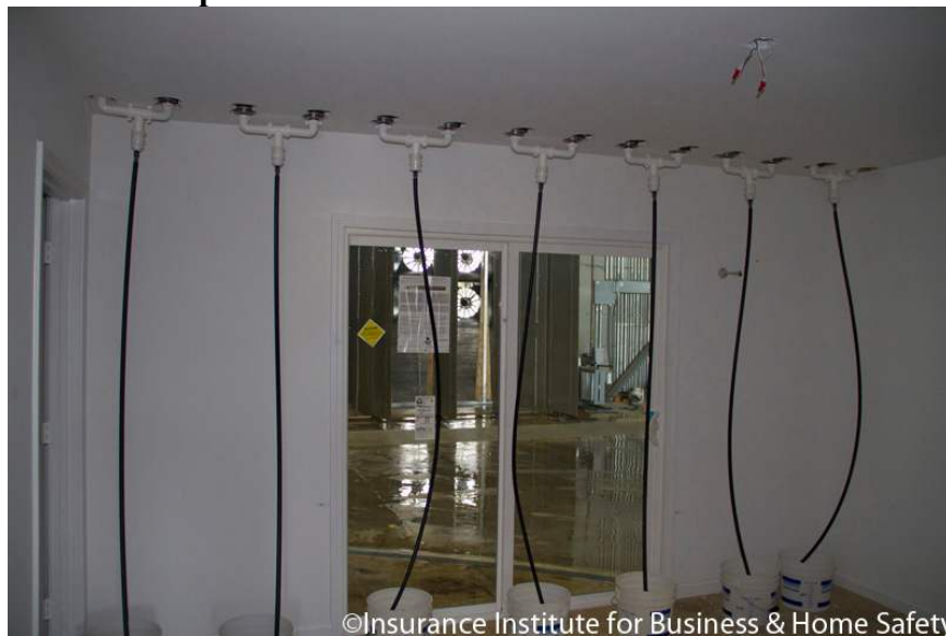
Figure 1. Photograph of water collection channels between ceiling trusses in duplex.
